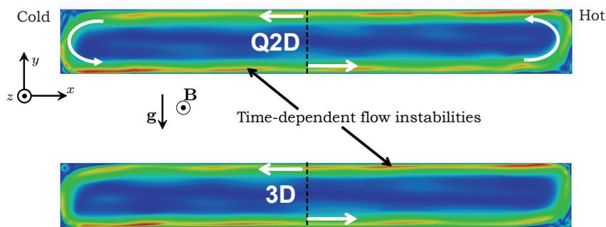
Fig. 4. Colored contours of the velocity magnitude in the vertical symmetry plane  $z = 0$  obtained by Q2D and 3D simulations for  $a = 1$ ,  $Gr = 10^8$ ,  $Pr = 0.015$ ,  $Ha = 1000$ ,  $c = 0$ .
