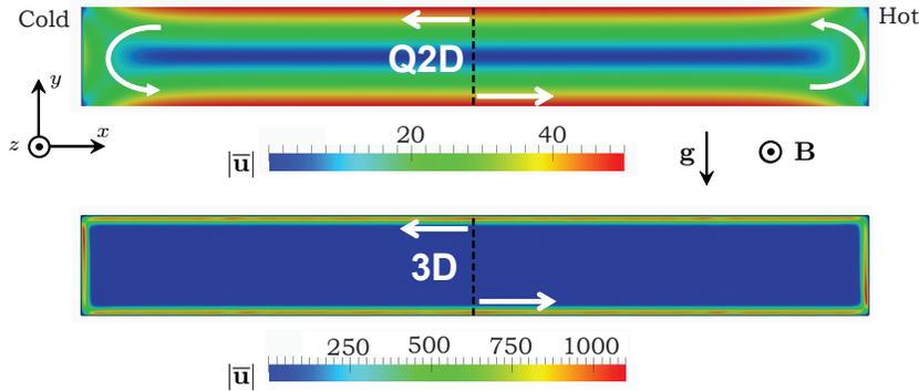
*Fig. 5.* Colored contours of the velocity magnitude in the vertical symmetry plane  $z = 0$  obtained by Q2D and 3D simulations for  $a = 1$ ,  $Gr = 10^8$ ,  $Pr = 0.015$ ,  $Ha = 1000$ ,  $c = \infty$ .
