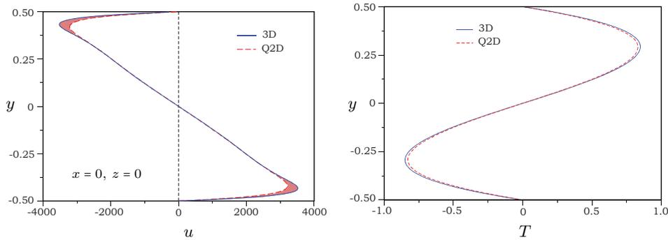
Fig. 3. Comparison of axial velocity and temperature along  $y$  at  $(x, z) = (0, 0)$  obtained by Q2D and 3D simulations for  $a = 1$ ,  $Gr = 10^7$ ,  $Pr = 0.015$ ,  $Ha = 1000$ ,  $c = 0$ .
