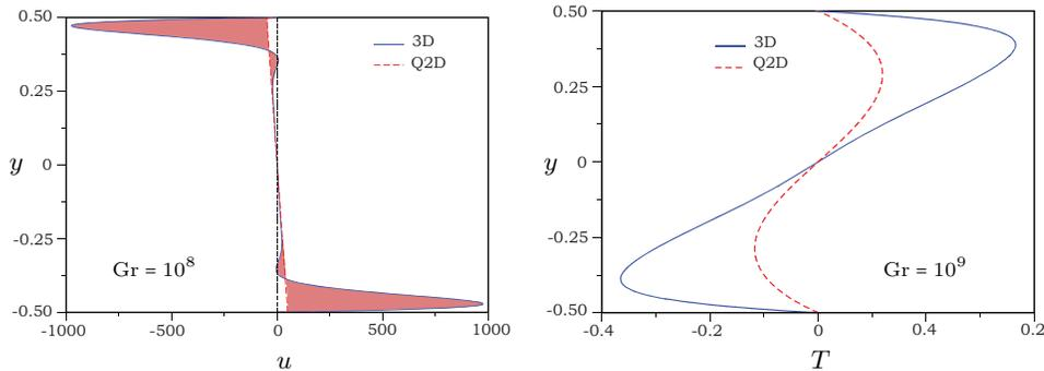
*Fig. 6.* Comparison of axial velocity and temperature along  $y$  at  $(x, z) = (0, 0)$  obtained by Q2D and 3D simulations for  $a = 1$ ,  $Pr = 0.015$ ,  $Ha = 1000$ ,  $c = \infty$ .
