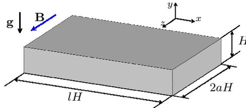
*Fig. 1.* Sketch of geometry and coordinates. The flat cavity, filled with liquid metal, is differentially heated at  $x/H = \pm 1/2$ , such that a mean axial temperature gradient  $G\hat{x}$  establishes. Top and bottom walls at  $y/H = \pm 1/2$  have temperature profiles that vary linearly between the values of the differentially heated walls. The other walls are adiabatic. The convective motion is damped by a horizontal magnetic field in the  $z$ -direction.
