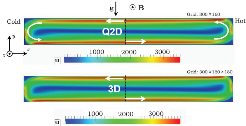
Fig. 2. Colored contours of the velocity magnitude in the vertical symmetry plane  $z = 0$  obtained by Q2D and 3D simulations for  $a = 1$ ,  $Gr = 10^7$ ,  $Pr = 0.015$ ,  $Ha = 1000$ ,  $c = 0$ .
